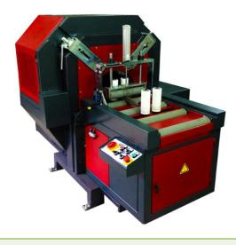
There are 4 profile centering rollers working with pneumatic system at the entrance. There is also 1 roller working with pneumatic system that presses the profile from the top.
