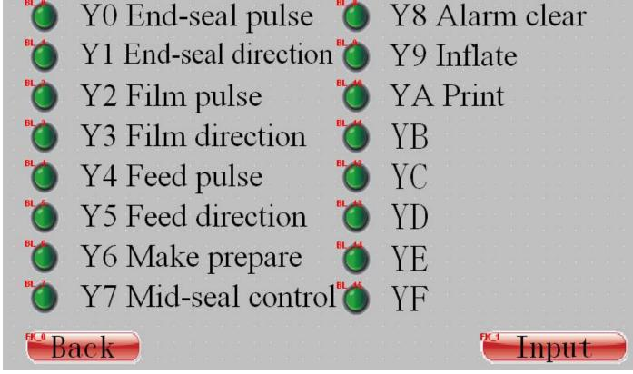
Input and output monitoring can display the input and output state, and to determine the electrical fault
