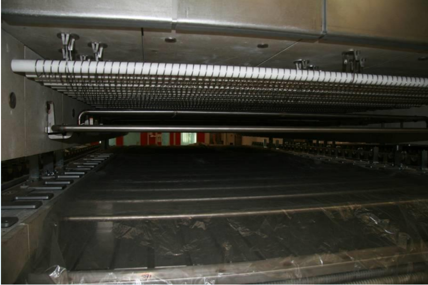
Top and bottom aspirator pipes into the heating tunnel
