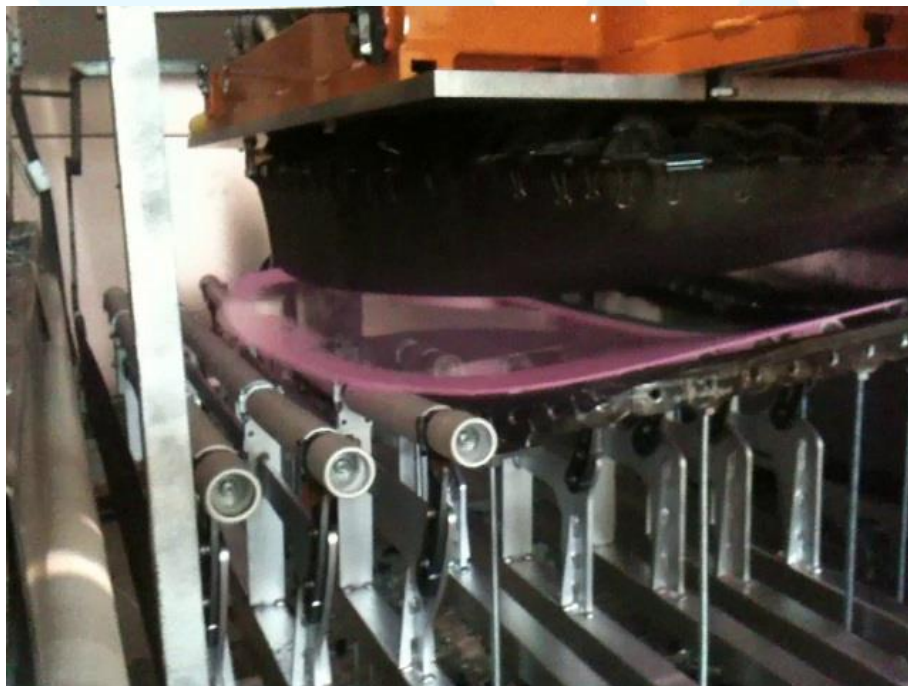
BSH+ gradually pre-bending process
