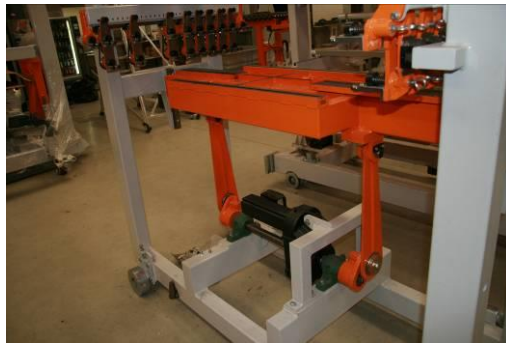
OH+ servomotor with cam for press ring movement
