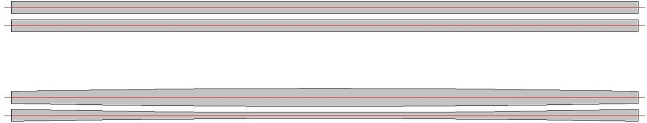
Secondary direction bending with flat and barreled rollers
