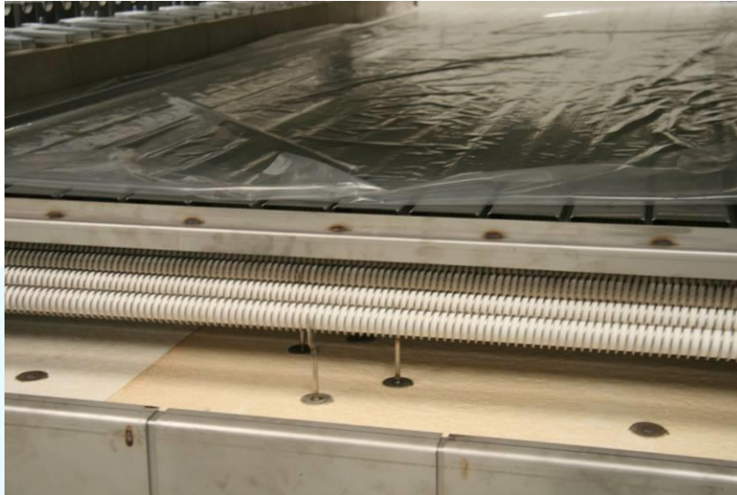
Bottom heating elements with steel covers
