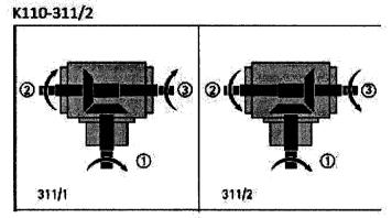
These are the two types. → it is more or less the same gearbox. The only difference are borings if not on both sides.
