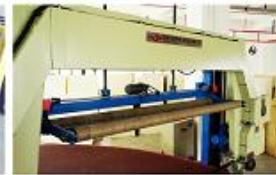
可选装固定式前后压辊 Optional the stationary front and back pressure roller
