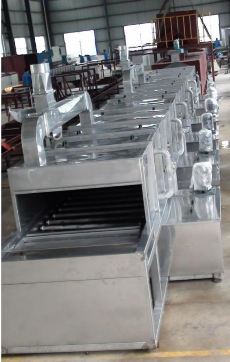
Desktop cleaning production line: electric power: 26KW Natural gas: 150,000 kcal (20 burners)
