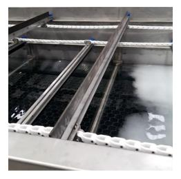
The system has been designed to treat wastewater flows with a very high load of suspended solids and other contaminants, which require a large flotation surface to ensure good flotation and separation of solids (up to 40kg of dry matter per m<sup>2</sup> can be treated).
