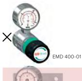
Single-stage, for inert, reactive, flammable and oxidizing gases and gas mixtures, purity max. 6.0, Inlet pressure 40 bar / 600 psi, Outlet pressure range 0.1 – 10.5 bar / 1 – 150 psi
