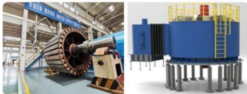
正在制造的3750kW, 25r/min人离心机电机 (图左为电机转子, 图右为三维模型) 3,750kW, 25r/min manned centrifuge motor being manufactured (motor rotor on the left picture, 3D model on the right picture)
