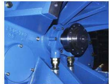
Fig. 24: Main oil pump
